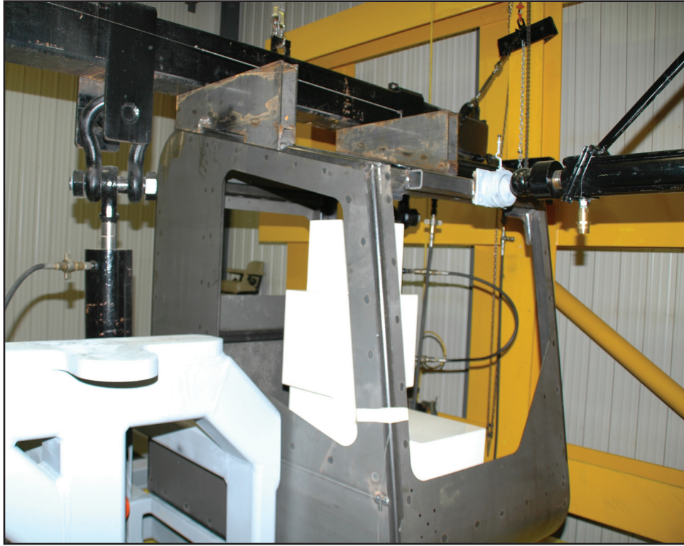
Photo of Custom Products' zero degree test lab with a cab enclosure during ROPS certification tests.
