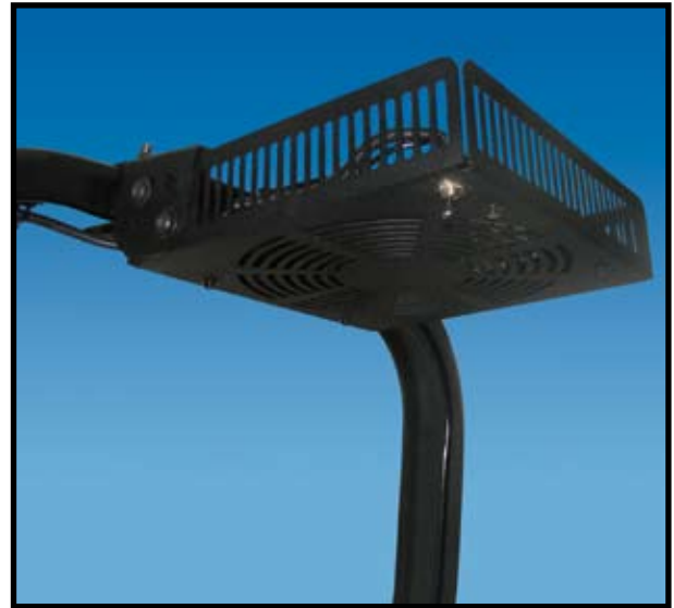
ROPS Mounted Cooling Fan
