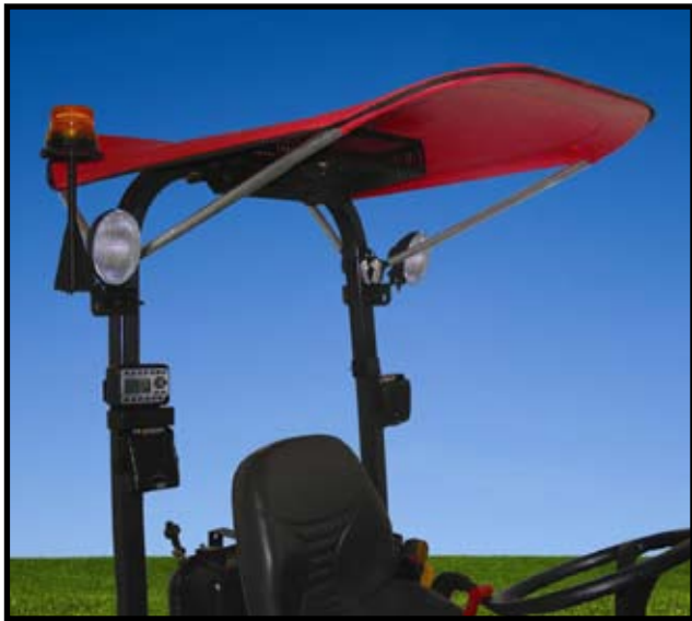
ROPS Mounted Accessories Including Cooling Fan
